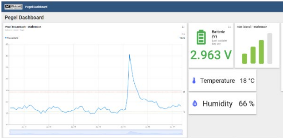
Figure 3: Dashboard prototype realized in Thingsboard 9 for visualization and analysis of measurement data with water level thresholds for generating alarm systems
