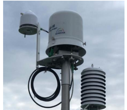
Figure 1: ASI-16/55 with radiation shield in the middle, left the pyranometer and right the temperature and humidity sensor
